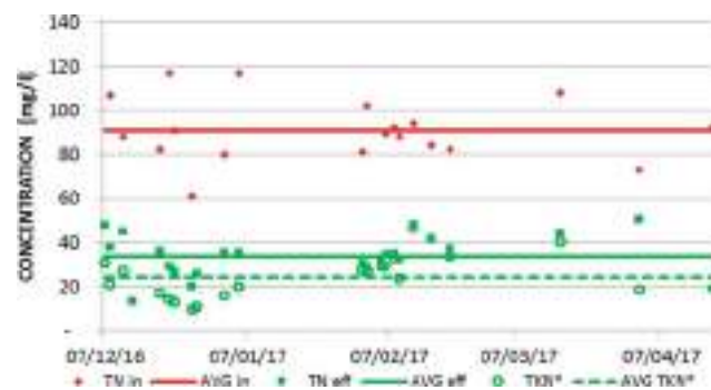
Fig. 1 TN and TKN concentration over time— influent and effluent. TKN* is a calculated value for total nitrogen analysis without the nitrate. It is a more relevant performance indicator for the MABR influence on the poorly aerated non-nitrifying pond to which it returns the treated wastewater.
