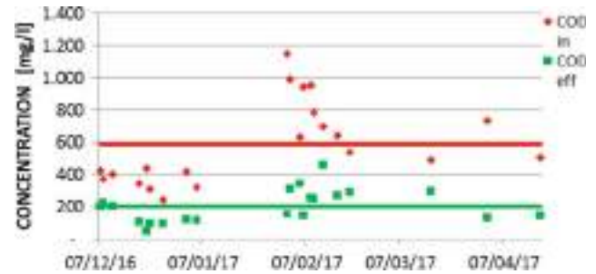
Fig. 2 COD influent and effluent over time
