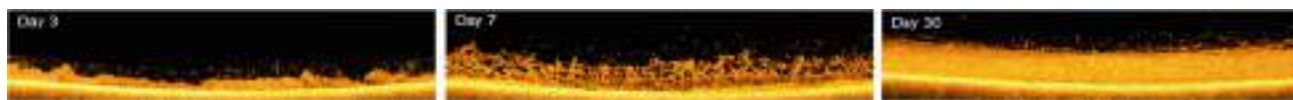
Fig. 1 Changes in biofilm morphology acquired by OCT scan over the time in submerged membrane bioreactor
