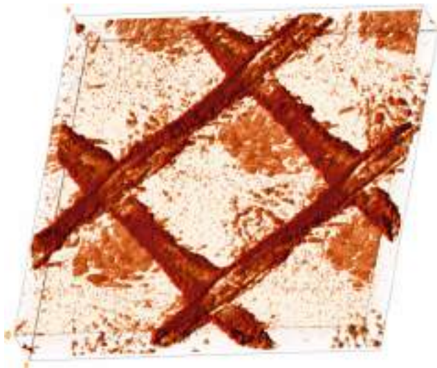
Fig. 2 3D rendered OCT image with biomass in spacer-filled channel
