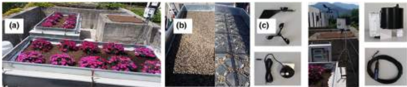
Fig. 1 a GR experimental test beds at University of Salerno, b drainage layer construction types, c the monitoring system
